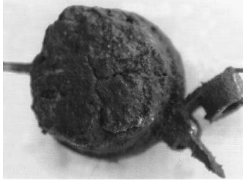
Fig. 3. The 58.5%:35%:6.5% PG:class C fly ash:lime composite exhibited severe degradation after 6 weeks saltwater submergence.
